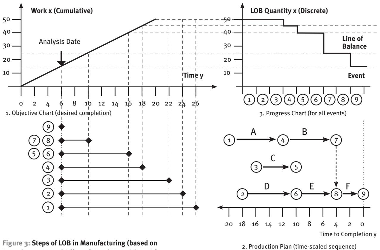
**Figure 3: Steps of LOB in Manufacturing (based on Lumsden, 1968 and Office of Naval Material, 1962).**
