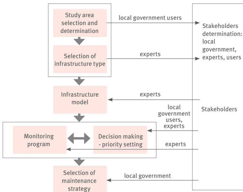
Figure 2: Maintenance decision making process flow diagram
