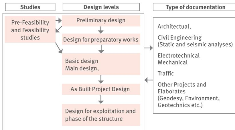
**Figure 2: Main levels of design and type of documentation according to the Law on Construction**
