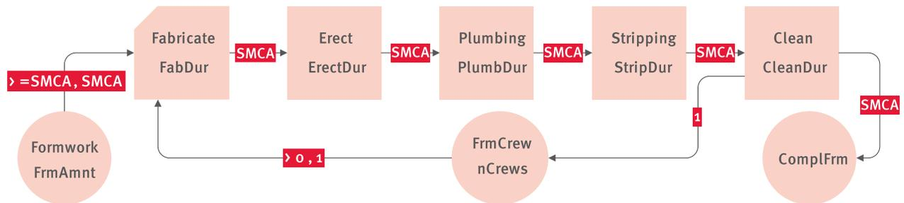
Figure 3. Generic simulation model for formwork operations.
