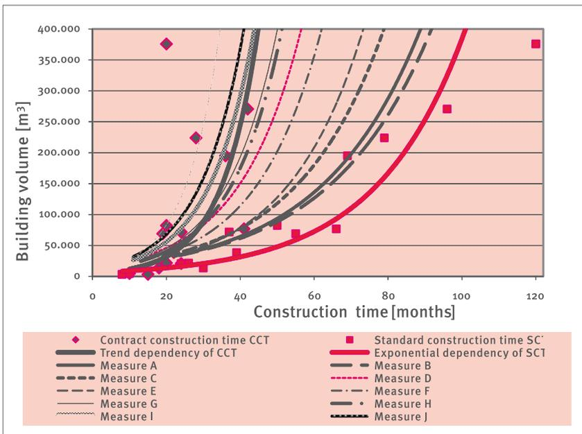
Figure 3. Impacts of the measures for construction time shortening in multifunctional buildings segment
