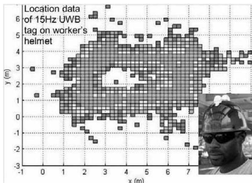
**Figure 4. Plan view of Circular Travel Path (Teizer et al. 2008)**
